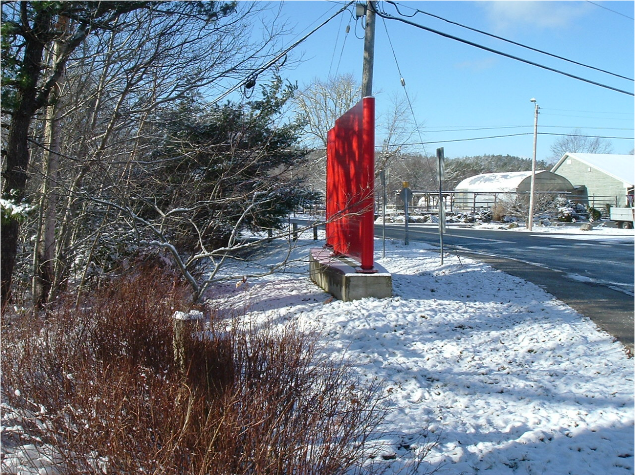
Figure 5. This is the view to the west, from a vehicle stopped in the Redding Driveway, when the front of the vehicle partly obstructs the sidewalk. Note that the Welcome Sign blocks the driver's view of part of Falls Lane, where vehicles need to stop for the stop sign. Look at this photo, and imagine what the driver's view would be, if the sign is moved to the south (left in this photo), with the edge of the sign foundation located at the edge of the large rock (which is hard to see in this photo – so look at Figure 4 to see where the rock is located).
